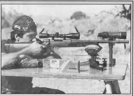
After subjecting the barreled action to deep cryogenic stress relief, the Steyr SSG-PIIK consistently shot 0.4 MOA groups off the bench at both 100 and 200 meters.
